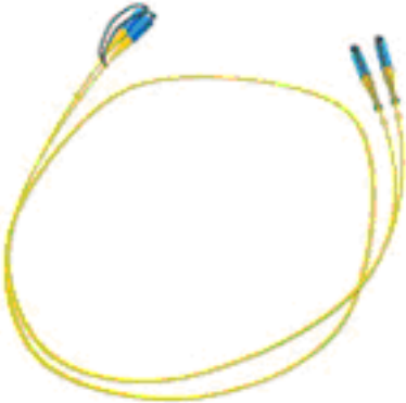
Fig 2.11. Crossing cable of duplex type; single mode SMF, SC-SC end
