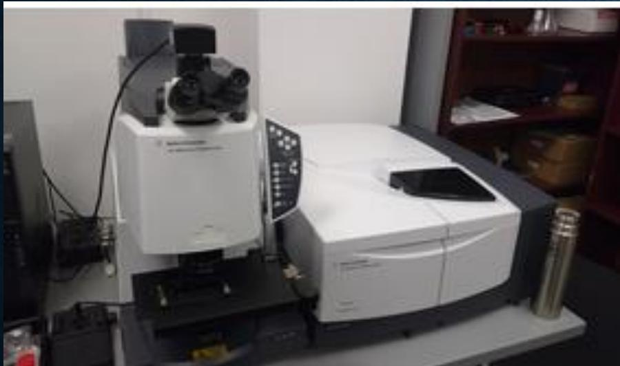
FTIR microscope (Agilent Technologies
